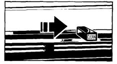
Move the Lock Lever to the right – the Clean position. The Oven HEAT-ING and ON Indicator Lights will come on.
