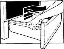
2. Lift back slightly and slide drawer all the way out.
