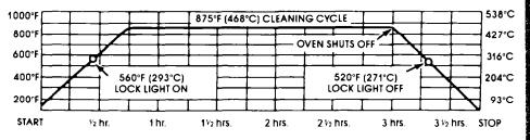
Notice that the heating stops when the 3-hour setting is up, but that it takes longer for the oven to cool down enough to unlock.
