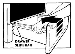
1. Fit ends of drawer slide rails into the drawer guides on both sides of opening.
