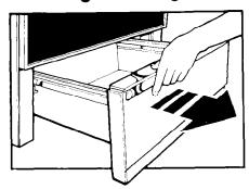
1. Empty drawer of any pots and pans before removing drawer. Pull drawer straight out to the first stop. Lift front and pull out to the second stop.
