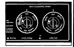
5. When baking is done, turn **both** the Oven Selector and Oven Temperature Control to OFF. The Oven HEATING and ON Indicator Lights will go OFF.
