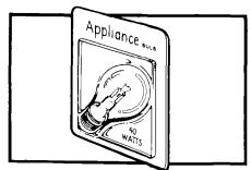
3. Remove the light bulb from its socket. Replace the bulb with a 40-watt appliance bulb.
