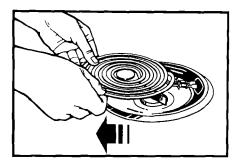
**3.** Pull the surface unit straight away from the receptacle.
