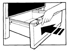
2. Lift drawer front and push in until metal stops on drawer slide rails clear white stops on drawer guides. Lift drawer front again to clear second stop and slide drawer closed.
