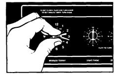
2. Let the Minute Timer Knob pop out. Turn clockwise until Minute Timer hand points to OFF. The clock setting will change if you push in the knob when turning.
