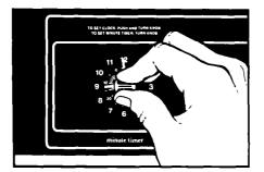
1. Without pushing it in, turn the Minute Timer Knob until the timer hand passes the setting you want.
