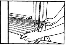
1. Position the rack(s) properly before turning on the oven. To change rack position, lift rack at front and pull out.
