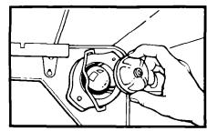
2. Remove the bulb cover in the back of the oven by pulling out and pushing the wire holder to the side.
