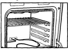
Position the rack before turning the oven on. See "Broil Chart" in the Cooking Guide or a reliable cookbook for recommended rack positions.
