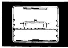
4. Put food in the oven. During baking, the elements will turn on and off to keep the oven temperature at the setting. The Oven HEATING Indicator Light will turn on and off with the elements.
