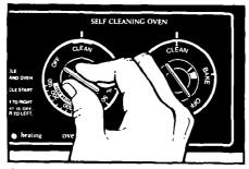
**1.** Set the Oven Selector and Oven Temperature Control on CLEAN.
