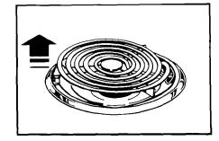
**2.** Lift the edge of the unit, opposite the receptacle, just enough to clear the element hold down clip and the reflector bowl.
