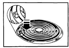
4. When terminal is pushed into the receptacle as far as it will go, push down the edge of the surface unit opposite the receptacle. The element hold down clip will keep the surface unit from moving around.
