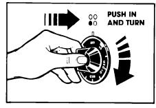
Control knobs must be pushed in before turning them to a setting. They can be set anywhere between HI and OFF.
