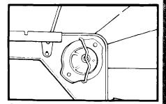
**4.** Replace the bulb cover and snap the wire holder in place. Plug in appliance or reconnect at the main power supply.
